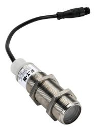
Eaton photoelectric sensor, tubular, threaded, 303 stainless steel housing, through-beam receiver, 250m sensing distance, 10-30 VDC operating voltage, dark-on, NPN/PNP, 4-wire, 4-pin M12 quick-disconnect.
