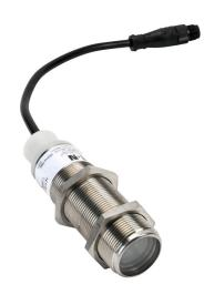
Eaton photoelectric sensor, tubular, threaded, 303 stainless steel housing, through-beam receiver, 250m sensing distance, 15-30 VDC/20-132 VAC operating voltage, light-on, solid state relay, 3-wire, 4-pin AC micro 1/2in-20 UNF thread.
