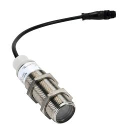
Eaton photoelectric sensor, tubular, threaded, 303 stainless steel housing, through-beam receiver, 250m sensing distance, 15-30 VDC/20-132 VAC operating voltage, dark-on, solid state relay, 3-wire, 4-pin AC micro 1/2in-20 UNF thread.
