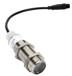
Eaton photoelectric sensor, tubular, threaded, retroreflective, visible red, 18m sensing distance, light-on, NPN/PNP, 4-wire, 4-pin M12 quick-disconnect.
