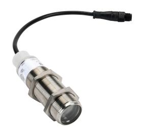
Eaton photoelectric sensor, tubular, threaded, retroreflective, visible red, 18m sensing distance, dark-on, NPN/PNP, 4-wire, 4-pin M12 quick-disconnect.
