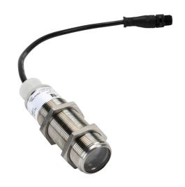
Eaton photoelectric sensor, tubular, threaded, retroreflective, visible red, 18m sensing distance, dark-on, solid state relay, 3-wire, 4-pin AC micro 1/2in-20 UNF thread.
