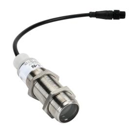
Eaton photoelectric sensor, tubular, threaded, polarized retroreflective, visible red, 10m sensing distance, light-on, NPN/PNP, 4-wire, 4-pin M12 quick-disconnect.
