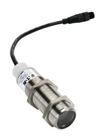
Eaton photoelectric sensor, tubular, threaded, polarized retroreflective, visible red light emission, 10m sensing distance, dark-on, NPN/PNP, 4-wire, 4-pin M12 quick-disconnect.
