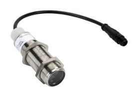
Eaton photoelectric sensor, tubular, threaded, polarized retroreflective, visible red light emission, 10m sensing distance, light-on, solid state relay, 3-wire, 4-pin AC micro 1/2in-20 UNF thread.
