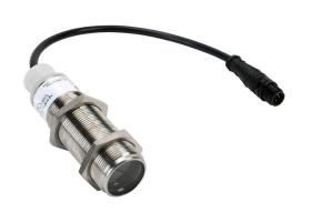
Eaton photoelectric sensor, tubular, threaded, polarized retroreflective, visible red, 10m sensing distance, light-on, solid state relay, 3-wire, 4-pin AC micro 1/2in-20 UNF thread.
