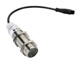
Eaton photoelectric sensor, tubular, threaded, polarized retroreflective, visible red light emission, 10m sensing distance, dark-on, solid state relay, 3-wire, 4-pin AC micro 1/2in-20 UNF thread.
