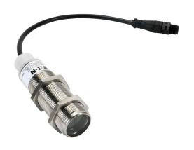
Eaton photoelectric sensor, tubular, threaded, polarized retroreflective, visible red, 10m sensing distance, dark-on, solid state relay, 3-wire, 4-pin AC micro 1/2in-20 UNF thread.
