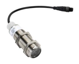
Eaton photoelectric sensor, tubular, threaded, diffuse with background suppression, 280mm sensing distance, light-on, NPN/PNP, 625 Hz switching frequency, 7in cable length, 4-pin M12 quick-disconnect.
