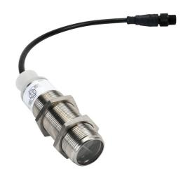
Eaton photoelectric sensor, tubular, threaded, diffuse with background suppression, 280mm sensing distance, dark-on, NPN/PNP, 625 Hz switching frequency, 7in cable length, 4-pin M12 quick-disconnect.
