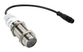
Eaton photoelectric sensor, tubular, threaded, diffuse with background suppression, 280mm sensing distance, light-on, solid state relay, 100 Hz switching frequency, 7in cable length, 4-pin AC micro 1/2in-20 UNF thread.
