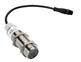
Eaton photoelectric sensor, tubular, threaded, diffuse with background suppression, 280mm sensing distance, dark-on, solid state relay, 100 Hz switching frequency, 7in cable length, 4-pin AC micro 1/2in-20 UNF thread.
