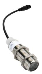
Eaton photoelectric sensor, tubular, threaded, diffuse with background suppression, 150mm sensing distance, light-on, NPN/ PNP, 625 Hz switching frequency, 7in cable length, 4-pin M12 quick-disconnect.
