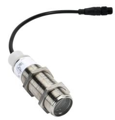
Eaton photoelectric sensor, tubular, threaded, diffuse with background suppression, 150mm sensing distance, dark-on, NPN/ PNP, 625 Hz switching frequency, 7in cable length, 4-pin M12 quick-disconnect.
