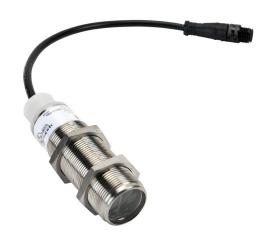
Eaton photoelectric sensor, tubular, threaded, diffuse with background suppression, 150mm sensing distance, light-on, solid state relay, 100 Hz switching frequency, 7in cable length, 4-pin AC micro 1/2in-20 UNF thread.
