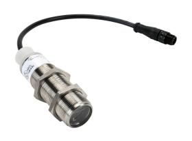
Eaton photoelectric sensor, tubular, threaded, diffuse with background suppression, 150mm sensing distance, dark-on, solid state relay, 100 Hz switching frequency, 7in cable length, 4-pin AC micro 1/2in-20 UNF thread.
