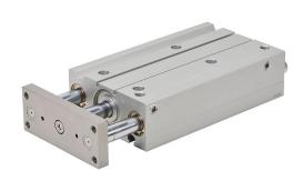
NITRA pneumatic cylinder, dual guide rod, 50mm bore, 20mm rod diameter, 200mm stroke, double acting, magnetic piston, universal mount.
