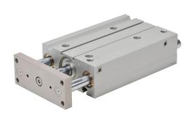
NITRA pneumatic cylinder, dual guide rod, 50mm bore, 20mm rod diameter, 175mm stroke, double acting, magnetic piston, universal mount.
