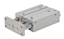
NITRA pneumatic cylinder, dual guide rod, 50mm bore, 20mm rod diameter, 150mm stroke, double acting, magnetic piston, universal mount.
