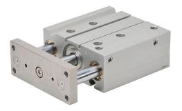
NITRA pneumatic cylinder, dual guide rod, 50mm bore, 20mm rod diameter, 100mm stroke, double acting, magnetic piston, universal mount.
