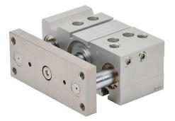
NITRA pneumatic cylinder, dual guide rod, 50mm bore, 20mm rod diameter, 25mm stroke, double acting, magnetic piston, universal mount.
