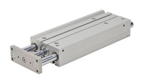
NITRA pneumatic cylinder, dual guide rod, 40mm bore, 16mm rod diameter, 250mm stroke, double acting, magnetic piston, universal mount.
