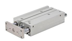
NITRA pneumatic cylinder, dual guide rod, 40mm bore, 16mm rod diameter, 175mm stroke, double acting, magnetic piston, universal mount.
