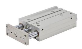
NITRA pneumatic cylinder, dual guide rod, 40mm bore, 16mm rod diameter, 150mm stroke, double acting, magnetic piston, universal mount.
