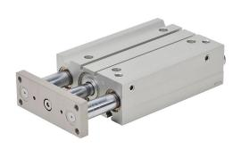
NITRA pneumatic cylinder, dual guide rod, 40mm bore, 16mm rod diameter, 125mm stroke, double acting, magnetic piston, universal mount.
