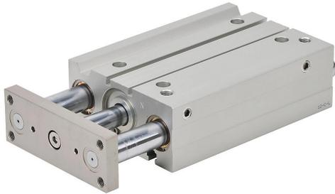
NITRA pneumatic cylinder, dual guide rod, 40mm bore, 16mm rod diameter, 125mm stroke, double acting, magnetic piston, universal mount.
