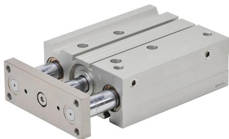
NITRA pneumatic cylinder, dual guide rod, 40mm bore, 16mm rod diameter, 100mm stroke, double acting, magnetic piston, universal mount.
