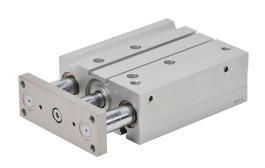
NITRA pneumatic cylinder, dual guide rod, 40mm bore, 16mm rod diameter, 100mm stroke, double acting, magnetic piston, universal mount.
