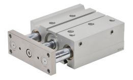
NITRA pneumatic cylinder, dual guide rod, 40mm bore, 16mm rod diameter, 75mm stroke, double acting, magnetic piston, universal mount.
