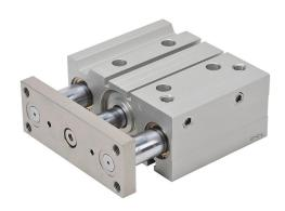
NITRA pneumatic cylinder, dual guide rod, 40mm bore, 16mm rod diameter, 50mm stroke, double acting, magnetic piston, universal mount.
