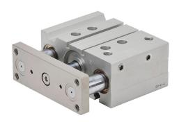
NITRA pneumatic cylinder, dual guide rod, 40mm bore, 16mm rod diameter, 40mm stroke, double acting, magnetic piston, universal mount.
