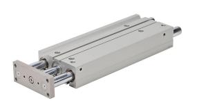
NITRA pneumatic cylinder, dual guide rod, 32mm bore, 16mm rod diameter, 250mm stroke, double acting, magnetic piston, universal mount.
