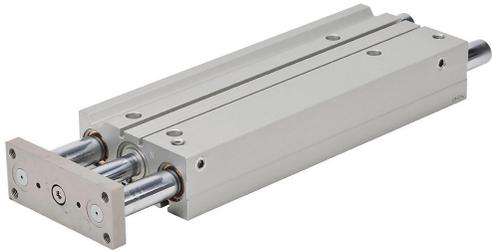
NITRA pneumatic cylinder, dual guide rod, 32mm bore, 16mm rod diameter, 250mm stroke, double acting, magnetic piston, universal mount.
