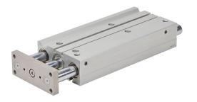
NITRA pneumatic cylinder, dual guide rod, 32mm bore, 16mm rod diameter, 200mm stroke, double acting, magnetic piston, universal mount.
