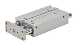
NITRA pneumatic cylinder, dual guide rod, 32mm bore, 16mm rod diameter, 150mm stroke, double acting, magnetic piston, universal mount.
