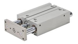
NITRA pneumatic cylinder, dual guide rod, 32mm bore, 16mm rod diameter, 125mm stroke, double acting, magnetic piston, universal mount.
