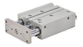
NITRA pneumatic cylinder, dual guide rod, 32mm bore, 16mm rod diameter, 100mm stroke, double acting, magnetic piston, universal mount.
