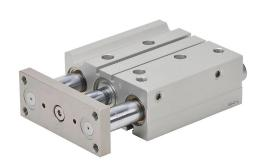
NITRA pneumatic cylinder, dual guide rod, 32mm bore, 16mm rod diameter, 75mm stroke, double acting, magnetic piston, universal mount.
