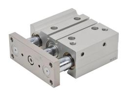
NITRA pneumatic cylinder, dual guide rod, 32mm bore, 16mm rod diameter, 50mm stroke, double acting, magnetic piston, universal mount.
