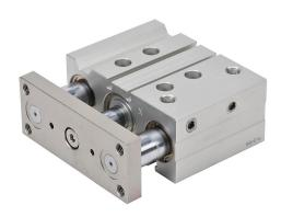
NITRA pneumatic cylinder, dual guide rod, 32mm bore, 16mm rod diameter, 40mm stroke, double acting, magnetic piston, universal mount.
