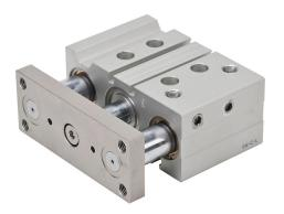
NITRA pneumatic cylinder, dual guide rod, 32mm bore, 16mm rod diameter, 30mm stroke, double acting, magnetic piston, universal mount.
