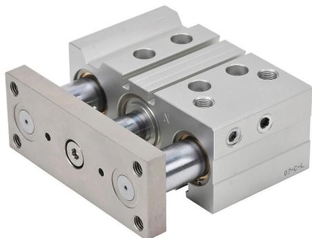
NITRA pneumatic cylinder, dual guide rod, 32mm bore, 16mm rod diameter, 25mm stroke, double acting, magnetic piston, universal mount.
