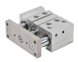
NITRA pneumatic cylinder, dual guide rod, 32mm bore, 16mm rod diameter, 25mm stroke, double acting, magnetic piston, universal mount.
