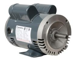
Marathon premium efficiency AC induction motor, general purpose, 3/4hp, 1-phase, 100-120/200-240 VAC, 1800rpm, ODP, NEMA 56C frame, rolled steel, C-face/rigid base mount.
