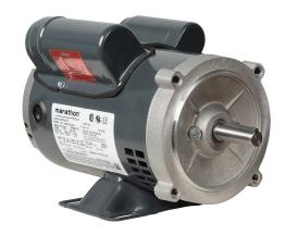
Marathon standard efficiency AC induction motor, general purpose, 1/2hp, 1-phase, 100-120/200-240 VAC, 1800rpm, ODP, NEMA 56C frame, rolled steel, C-face/rigid base mount.
