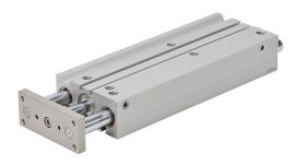
NITRA pneumatic cylinder, dual guide rod, 25mm bore, 12mm rod diameter, 200mm stroke, double acting, magnetic piston, universal mount.
