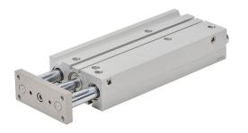
NITRA pneumatic cylinder, dual guide rod, 25mm bore, 12mm rod diameter, 175mm stroke, double acting, magnetic piston, universal mount.
