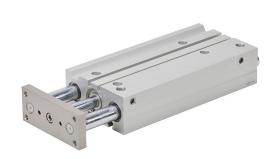
NITRA pneumatic cylinder, dual guide rod, 25mm bore, 12mm rod diameter, 150mm stroke, double acting, magnetic piston, universal mount.
