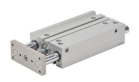
NITRA pneumatic cylinder, dual guide rod, 25mm bore, 12mm rod diameter, 125mm stroke, double acting, magnetic piston, universal mount.
