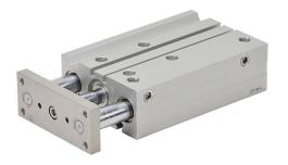
NITRA pneumatic cylinder, dual guide rod, 25mm bore, 12mm rod diameter, 100mm stroke, double acting, magnetic piston, universal mount.
