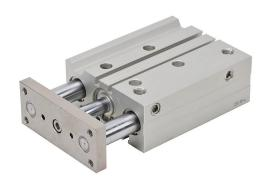
NITRA pneumatic cylinder, dual guide rod, 25mm bore, 12mm rod diameter, 75mm stroke, double acting, magnetic piston, universal mount.
