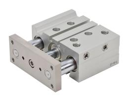
NITRA pneumatic cylinder, dual guide rod, 25mm bore, 12mm rod diameter, 30mm stroke, double acting, magnetic piston, universal mount.
